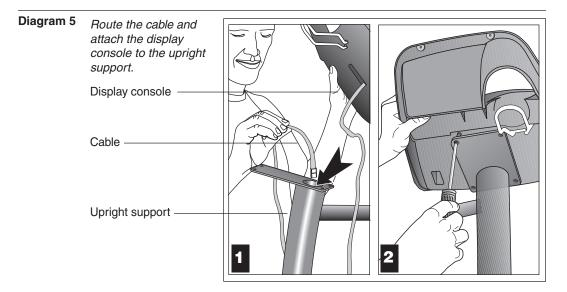
5. **Prepare for the attachment of the upright support to the base assembly.** Diagrams 5 and 6. Remove the four Phillips-head screws (D), two bolts (G), and two washers (H) from the Hardware kit. Place one washer (H) on each of the two bolts (G). Keep the fasteners together.
